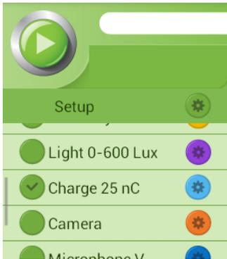
6. Tap the Setup button to calibrate or change the sensor's range
