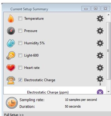
5. Click Full Setup, located at the bottom of the Current Setup Summary window to program the data logger's range, sample rate, number of samples, units of measurement, and other options.
