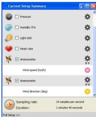
5. Click Full Setup, located at the bottom of the Current Setup Summary window to program the data logger's sample rate, number of samples, units of measurement, and other options
