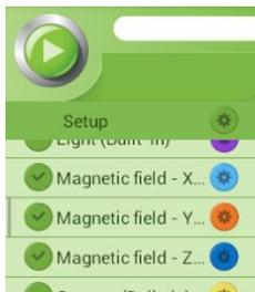
6. Make sure the icon next to the axis you want to measure is checked (  ) to enable it for logging
