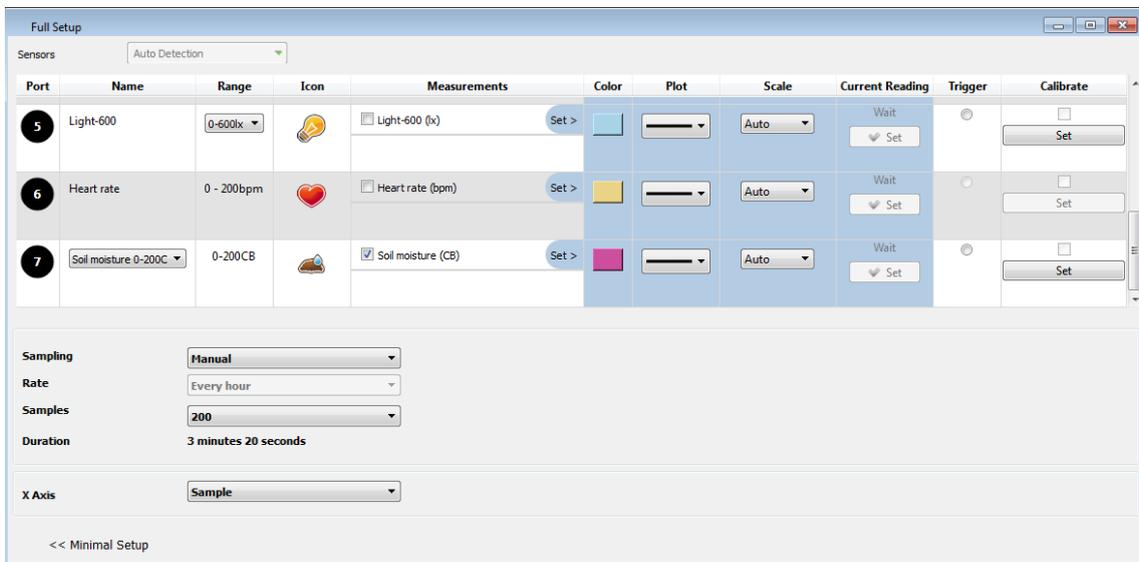
6. In Full Setup, you will be able to program the data logger’s sample rate, number of samples, units of measurement, and other options
